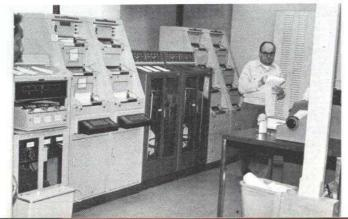
The Communication Center's teletypewriter patch panel allows duty operators to patch in alternate teletypewriter machines and the INTELSAT Operations center teletypewriter to any earth station it chooses for direct communications. Panel is also used for retrieving satellite pointing data from the Clarksburg, Md., computer.
