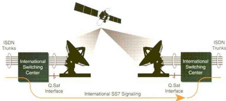
Q.Sat will enable satellite networks to manage their internal capacity more efficiently and improve the quality of service for calls routed on satellite circuits.
