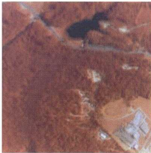
Magnified portions of a multispectral image of an airfield which has been compressed at 40:1 using spectral compression in conjunction with discrete cosine transform. The three-band composite images of the original (left) and compressed/decompressed (right) images are virtually indistinguishable.
