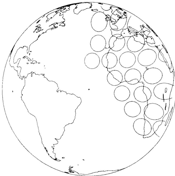
Figure 19. Beams Generated by Each Individual Feed
